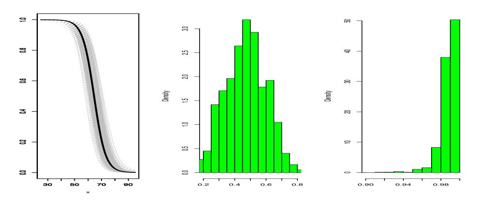
Predictive  $\Pr(Y = 1 | x) = \int \Pr(Y = 1 | x, \alpha, \beta) \pi(\alpha, \beta | \text{data})$ , predictions of failure probability at 65°F and 45°F.
