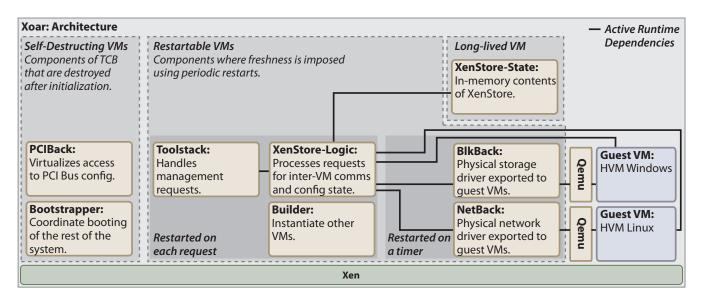
Figure 2: Architecture of Xoar. The figure above shows all the classes of service VMs along with the dependencies between them. For clarity, ephemeral dependencies (e.g., between the Builder and the VMs that it builds) are not shown. As suggested in the figure, a Qemu service VM is instantiated for the lifetime of each guest.
