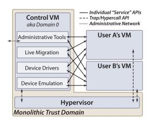
Figure 1: The control VM is often a full operating system install, has privilege similar to the hypervisor, and offers multiple services over numerous interfaces to guest VMs.
