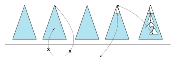
Figure 6: Trees in one level. The current level may call into the lower level, but no calls from the lower level may come into the current level. The level of an object is determined by the class that transitively owns the object, not by the object's type.
