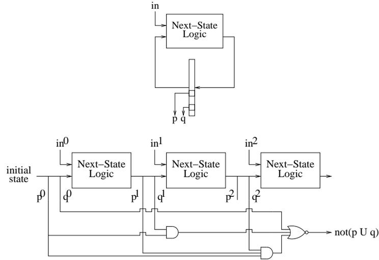
**Fig. 1.** Converting a Temporal Property to a Combinational One. To verify  $pUq$  over three clock cycles on a sequential circuit, we can unroll the circuit three times and create a combinational circuit whose output is true for any counterexample sequence.
