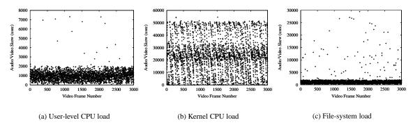
Figure 5: Audio/Video Skew on Linux-SRT with user-level CPU load, kernel CPU load and file-system load.
