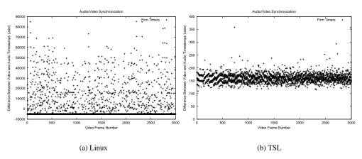
Background load copies a 8 MB buffer from user level to a file with a single write call. Note that the two figures have different scales, and that the maximum skew in Figure (b) is much smaller than in Figure (a).
