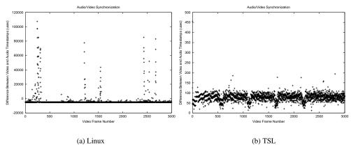
Background load repeatedly copies a compiled Linux kernel sources directory recursively and then flushes the file system. Note that the two figures have different scales, and that the maximum skew in Figure (b) is much smaller than in Figure (a).
