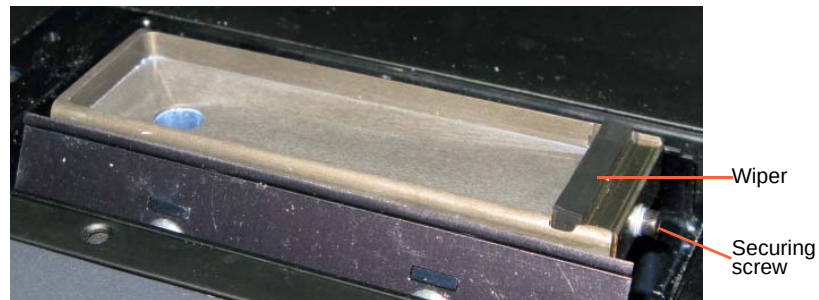
Figure 7-23: Wiper and excess-material drain
