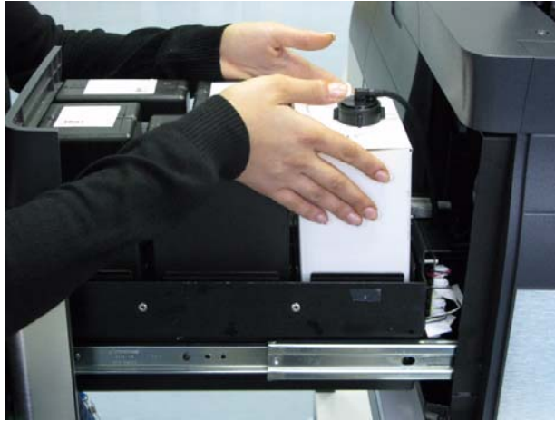
Figure 7-71: Removing the waste container
