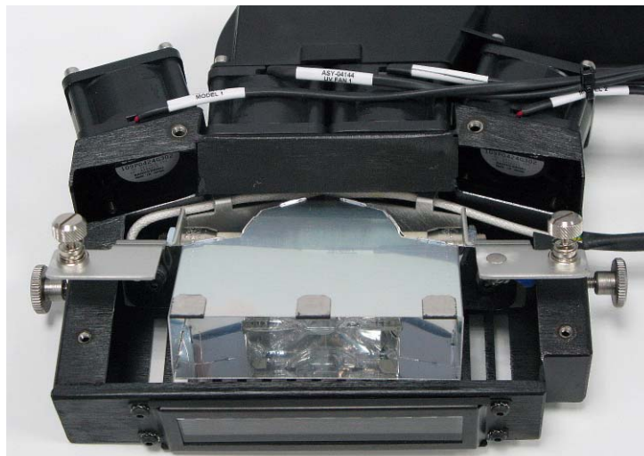
Figure 7-65: Removing the UV reflector from the UV assembly
