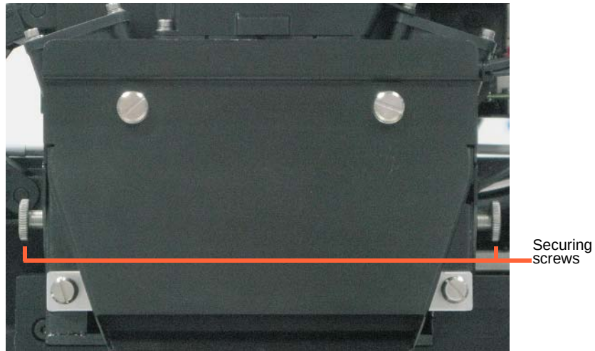
Figure 7-28: UV-lamp-assembly securing screws
