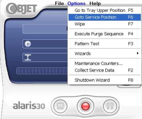
The screenshot shows the control panel interface with the 'Options' menu open. The menu items are: Go to Tray Upper Position (F5), Goto Service Position (F6), Wipe (F7), Execute Purge Sequence (F4), Pattern Test (F3), Wizards, Maintenance Counters..., Collect Service Data (F2), and Shutdown Wizard (F8). The 'Goto Service Position' option is highlighted in blue. Below the screen are three physical buttons: a square stop button, a red emergency stop button, and a vertical bar pause button.
