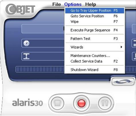
The screenshot shows the control panel interface with the 'Options' menu open. The menu items are: Go to Tray Upper Position (F5), Goto Service Position (F6), Wipe (F7), Execute Purge Sequence (F4), Pattern Test (F3), Wizards, Maintenance Counters..., Collect Service Data (F2), and Shutdown Wizard (F8). The 'Go to Tray Upper Position' option is highlighted in blue. Below the screen are three physical buttons: a square stop button, a red emergency stop button, and a vertical bar pause button.
