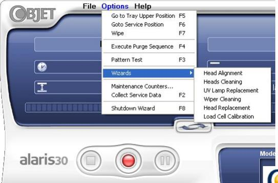
The screenshot shows the control panel interface with the 'Options' menu open and 'Wizards' expanded. The sub-options are as follows:
