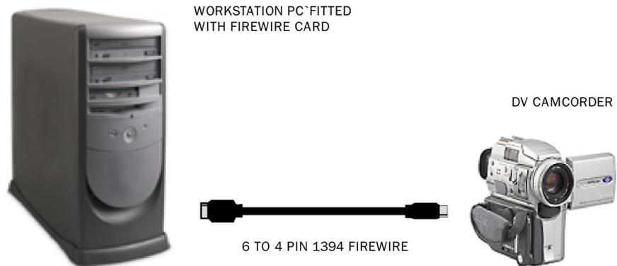
When using a DV Camcorder, you can connect it using a Firewire cable directly to the WorkStation PC Firewire port. A PCI 1394 Firewire card must be installed in the WorkStation PC.
