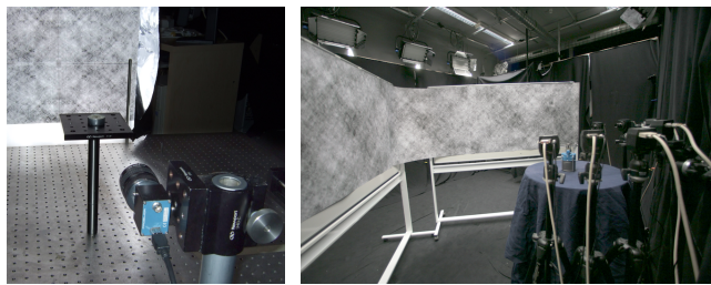
Figure 7: The single camera setup (left) and the camera array (right) that we use for acquisition.
