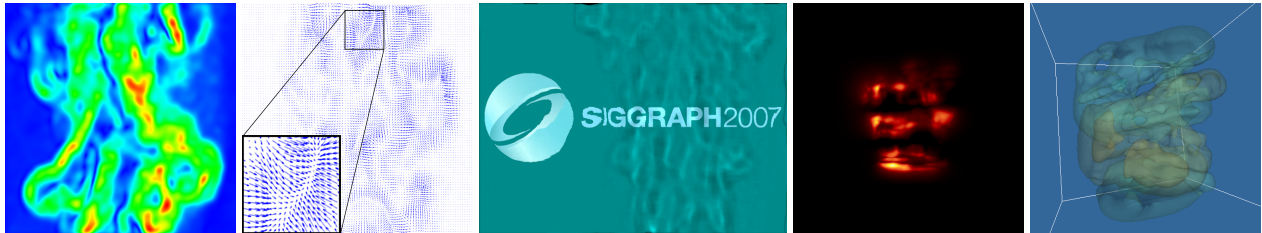
Figure 1: Measurements of the refractive index field caused by rising hot air from a gas burner. Far left: magnitude of refraction for each pixel in one view. Center left: vector field of 2D displacements. Center: distortion measurements from one view are used as an environment matte to distort the background, data from another view is used to cast a caustic (shadowgraph). Center right: maximum intensity projection volume rendering of a 3D refractive index field recovered with tomography from 8 views. Far right: volume rendering of the 3D reconstruction.
