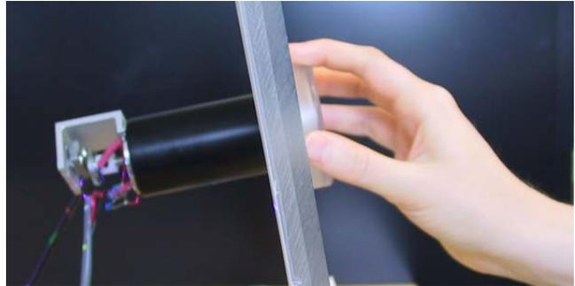
Figure 1: Haptic knob embedded into an acrylic graphical rear-projected display surface
