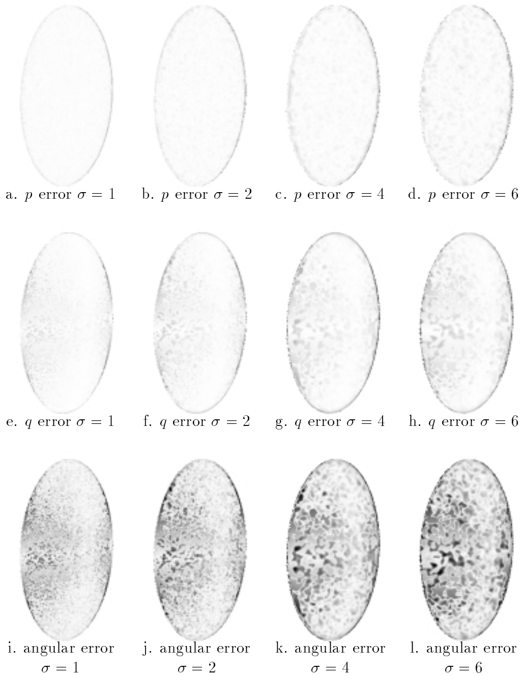
Figure 7.52: (a)-(e) are p error maps of the surfaces recovered from synthetic images of the different noise levels. (f)-(h) are q error maps of the recovered surfaces. (i)-(l) are angular error maps of the recovered surfaces.
