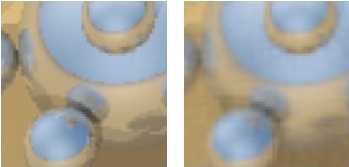
Figure 10: Original (left) and Reconstruction from 4-Dimensional Wavelet Coefficients (right)
