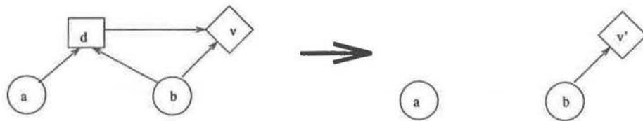
Figure 6.8: An illustration of decision node removal:  $d$  is removed by maximization
