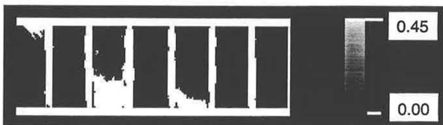
Figure 6.2: Reconstruction from successive POCS iterations incorporating the assumption that pixels are either air ( \mu = 0\text{cm}^{-1} ) or plexiglass ( \mu = 0.45\text{cm}^{-1} ).
