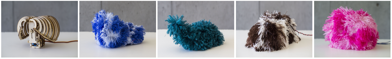
(a) RibBit: A CuddleBit that looks like a set of ribs. (b) FlexiBit: A Bit whose stomach "breaths" via a servo. (c) FlappyBit: A Bit with an appendage that flaps up and down via a servo. (d) VibroBit: A Bit that vibrates via an eccentric mass motor. (e) BrightBit: A Bit whose eyes light up via an LED.
