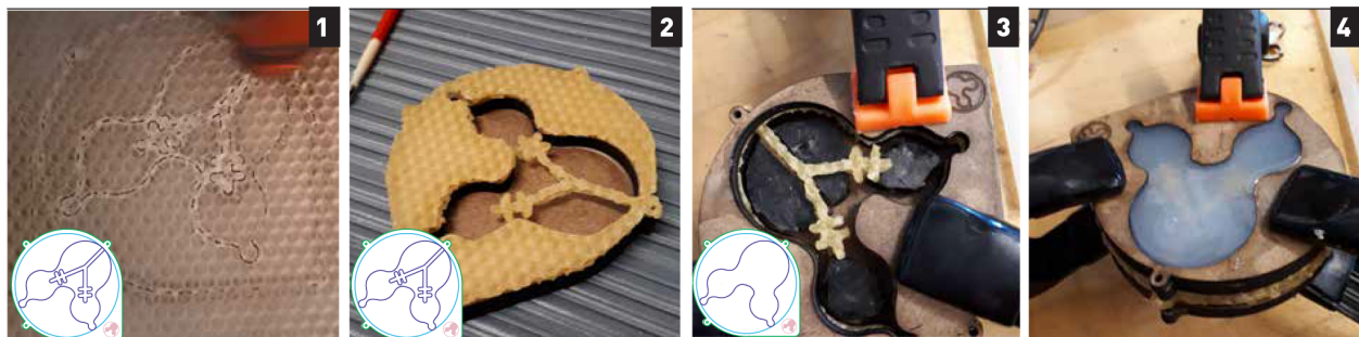
Figure 3.5: Steps to creating an actuated sensate object. (1) Laser-cut beeswax air channels. (2) Stack the air channels with the other layers to elevate them to the right height. (3) Place sensing pads. (4) Cure silicone around everything.
