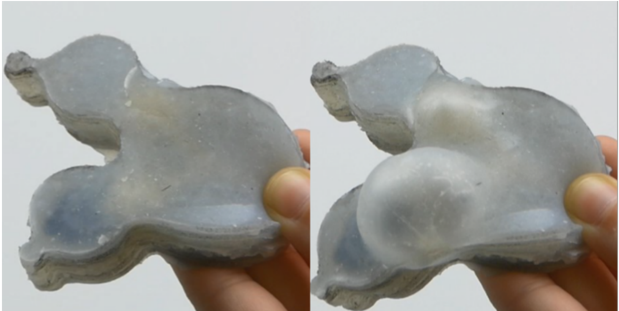
Figure 3.6: The final product of our actuator casting demonstration, showing the cast air channels being inflated.
