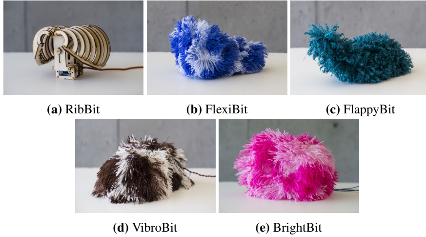
Figure 4.3: The 1-DOF CuddleBit robots used in the Voodle co-design study: (a) RibBit: A CuddleBit that looks like a set of ribs; (b) FlexiBit: A Bit whose stomach “breaths” via a servo; (c) FlappyBit: A Bit with an appendage that flaps up and down via a servo; (d) VibroBit: A Bit that vibrates via an eccentric mass motor; (e) BrightBit: A Bit whose eyes light up via an LED.
