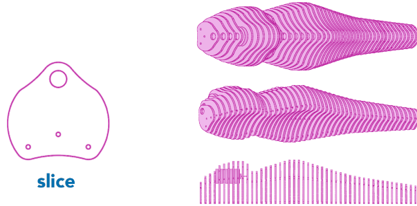
Figure 3.5: SpineBit design system. The whole robot is built off of configurations of a single slice (shown) which is defined by parameterized curves. By defining key slices and interpolating between them, a new robot shape can be produced.
