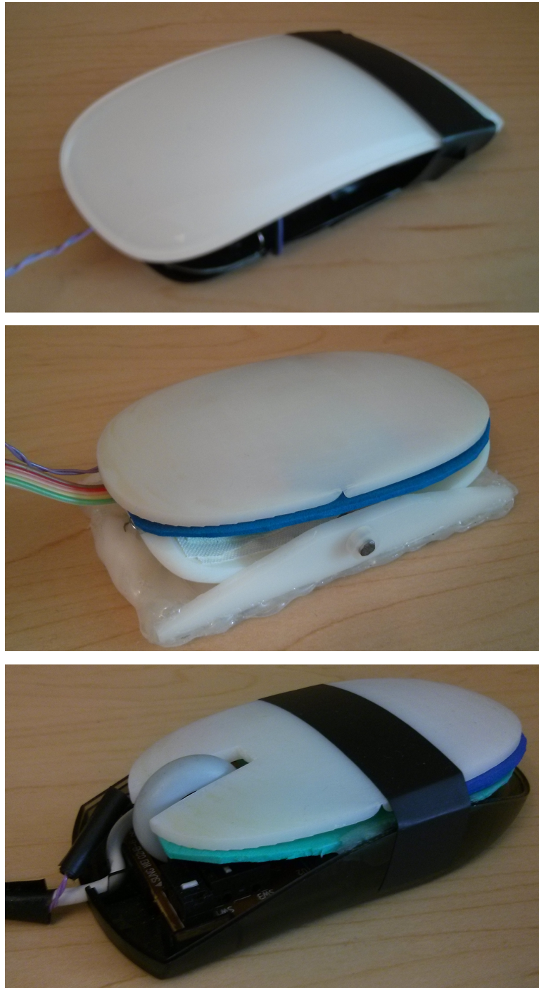
Figure 5.1: Image of the three prototypes used in the study: Touch, Tilt, Wheel/Click+Drag (both in one prototype).
