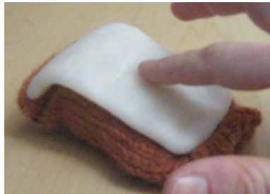
Figure 3.2: Early physical prototype: created out of POLYMORPH, knitted wool and stuffing.
