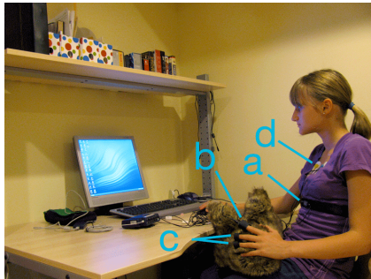
Image 1: User demonstrating possible physiological sensors: respiration rate (a), blood volume pulse (b), skin conductance (c), ECG (d).
