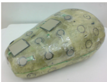
Figure 2.2: Touch sensors on the Haptic Creature’s surface
