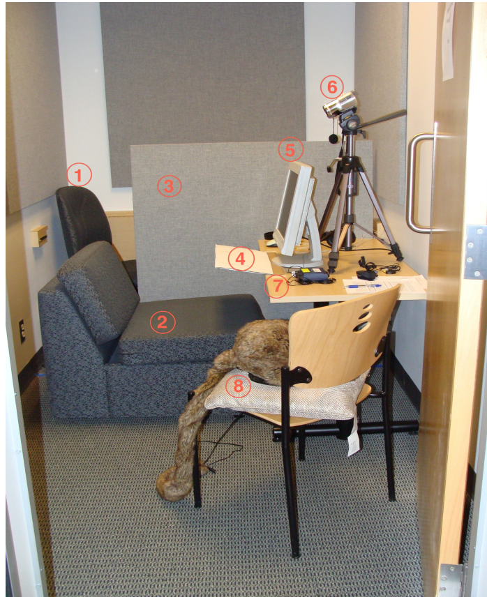
Figure 8.2: Study 2 - room setup. 1. facilitator's seat: during the trials the seat was completely behind the partition and invisible to the participant. 2. participant's seat. 3. office partition: this partition separated out the facilitator and the participant. 4. a white thick sheet of paper: this sheet covered the robot when participants kept it on their laps to minimize the possibility of visual interaction with the Haptic Creature. 5. participant's screen. 6. video camera. 7. Though Technology encoder. 8. the Haptic Creature and its cushion: during the baseline trials robot together with the cushion were placed on the ground out of participant's sight.
