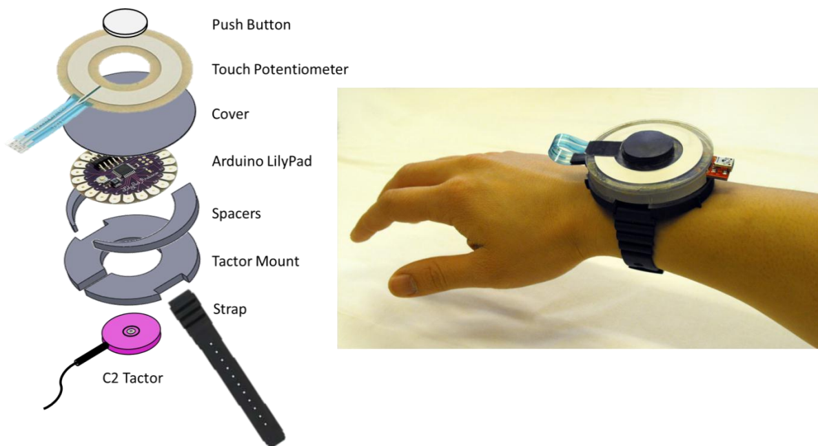
Figure 16. Exploded view and photo of wrist-worn navigational device and haptic display.
