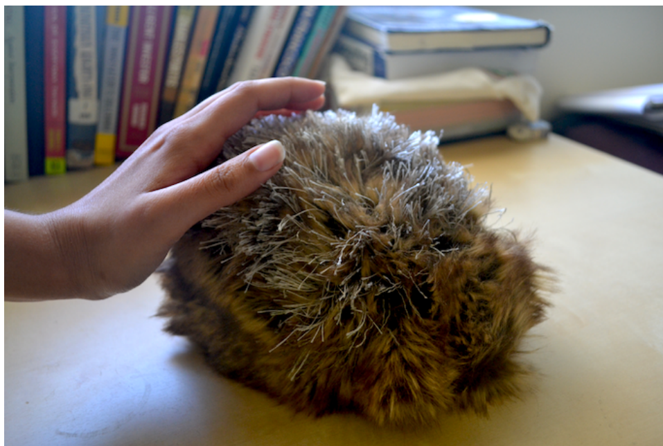
Figure 4.1: Hand stroking the touch-sensing creature prototype. Prototype is equipped with conductive fur and piezoresistive fabric pressure sensing, and sized \sim 15 \times 20 cm.
