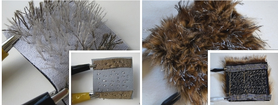
Figure 3.3: Perner-Wilson and Satomi’s conductive thread stroke sensor [13] (left), our conductive fur touch and gesture sensor (right).
