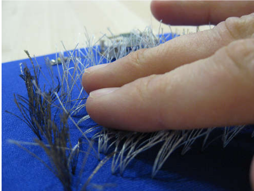
Figure 2.2: Perner-Wilson and Satomi’s conductive thread stroke sensor [13].
