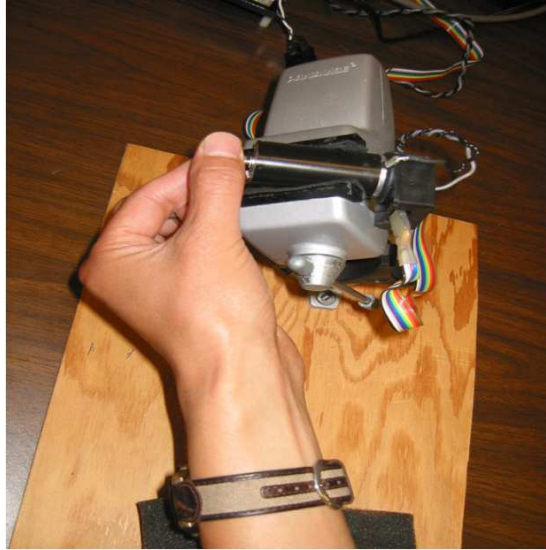
Figure 3-5 Participants held a haptically enabled knob through which haptic phonemes were displayed (Same as Figure 2-1)
