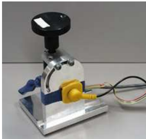
Figure 2-10 Direct drive haptic display: A knob mounted on the shaft of a DC coreless motor equipped with an optical encoder allowed recording and reproduction of haptic sensations.
