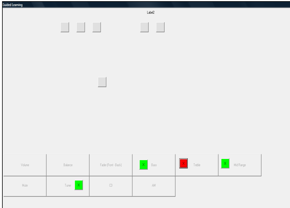
Figure 3-15 Guided learning and testing phase GUI. In training, participants tested their knowledge of the signals' meanings and received feedback as to their placement of the tactile signal tiles (green for correct placements, red for incorrect). Placement feedback was not given during the Test Phase.
