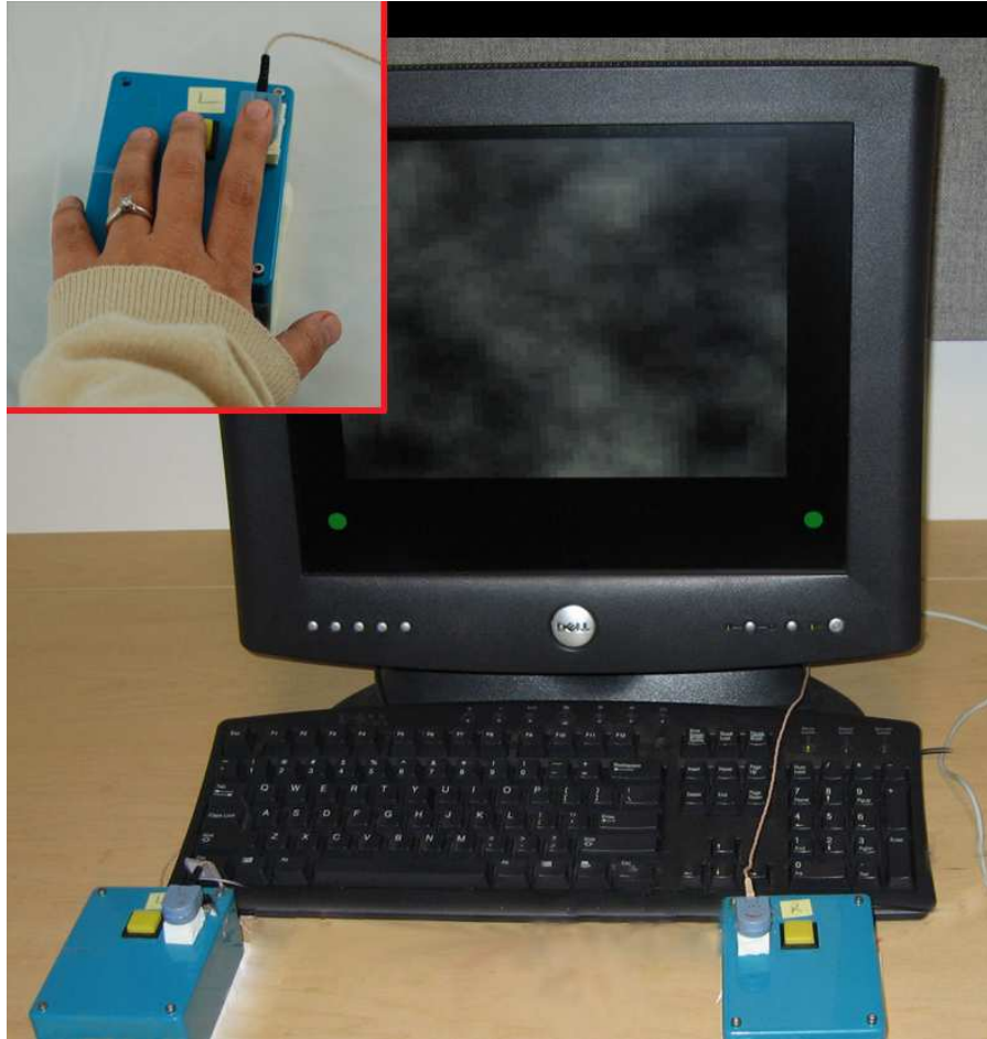
Figure 5-9 Physical setup. Participants placed one hand on each haptic display box and viewed the maze on the computer screen. The index fingers rested on the voice coil transducers (blue, mounted on blue boxes) to receive the haptic navigation cue; the middle fingers used the yellow response buttons. An oscillating motor providing background haptic noise is attached to the inside of each display box (not visible here). Not shown in this picture were two foam pads supporting wrists and forearms.
