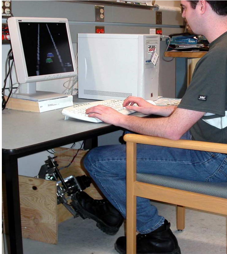
Figure 5-1 Setup. “Driver” at simulator with force feedback pedal.
