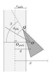
Fig. 3. Components of the potential field guidance method.  $\phi$  is the desired vehicle heading.
