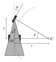
Fig. 2. Schematic of vehicle dynamics: the shaded area represents the vehicle. Tires are shown here for clarity, but are not rendered during the simulation.  $\theta$  is the current vehicle steering angle.
