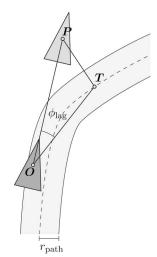
Fig. 4. Components of the look-ahead guidance method.  $\phi$  is the desired vehicle heading.
