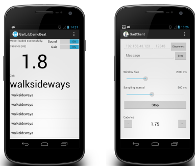
Figure 3. Left: the example app showing the current cadence and gait. Right: a demo app sending cadence via network with parameter control.
