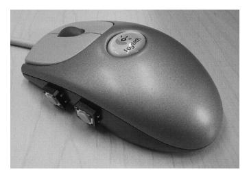
Fig. 4. Modified logitech iFeel mouse with thumb buttons.
