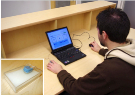
Figure 2: Experimental setup. The inset shows the vibrotactile actuator used in this experiment.
