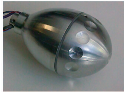
Fig. 4. Aladdin: a doorknob that communicates information to users about a common physical space through visual gesture and sound at a distance, and forces, vibrations and heat when in contact [64].
