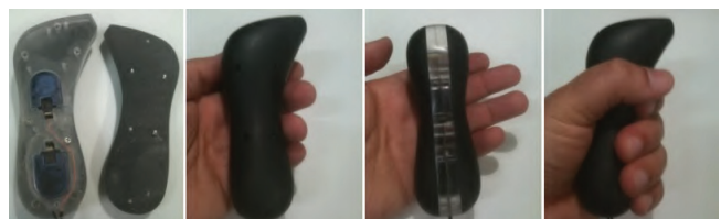
Figure 2. The handle designed to contain the VT transducers. From left to right: Handle opened to show the actuators, lateral view, rear view and grip used for last task in the study.
