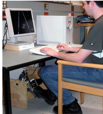
Figure 1: Setup. "Driver" at simulator with force feedback pedal.
