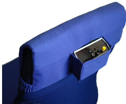
Fig. 3. Electronics unit located on the backrest of the chair
