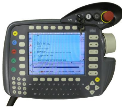
Figure 1. An example teach pendant (Kuka LWR controller). Such interfaces are ill-suited for human-robot collaborative work.
