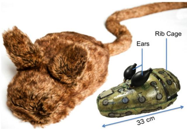
Fig. 1. The Haptic Creature (photo: Martin Dee) and its underlying structure. Key elements shown are a fiberglass shell  $\sim 33$  cm in length and covered with an array of touch sensors, stiffenable ears, and a moving rib cage that simulates breathing. Overall weight is  $\sim 2.5$  kg [1]. Simulated breathing was used in the study reported here.
