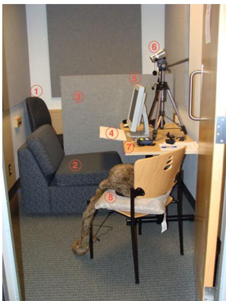
Fig. 3. Room setup. 1. Facilitator's seat: fully behind partition during trials. 2. Participant's seat. 3. Office partition. 4. Visual occlusion sheet. 5. Participant's computer screen. 6. Video camera. 7. Thought Technology encoder. 8. Haptic Creature and its cushion.
