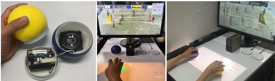
Fig. 1. External and internal views of the ball-type haptic device and practical examples.
