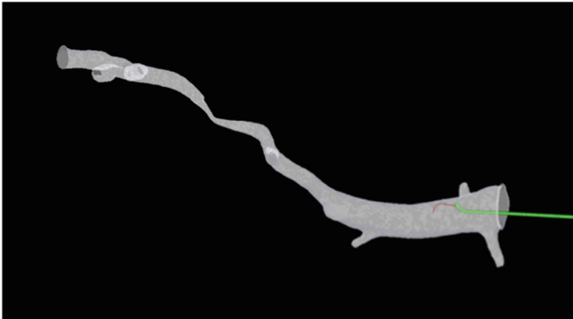
Fig. 4. 3D generated virtual environment with simulated vasculature and set of guidewire and catheter
