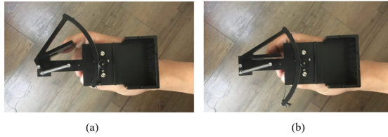
Fig. 2. The handset of spatial haptic feedback has force feedback mechanism for operator's pinch (between the thumb and forefinger).
