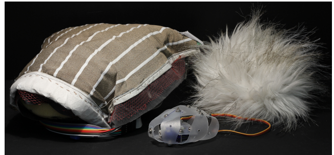
Figure 1: Three CuddleBits in various sizes and stages of dress. From Left to Right: (a) Large CuddleBit fitted with a fabric touch sensor; (b) Small CuddleBit skeleton; (c) Medium CuddleBit in a faux fur coat.
