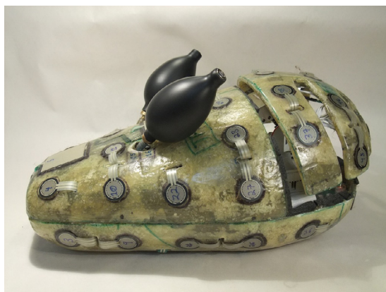
Fig. 3. Robot surface showing placements of 56 force sensing resistors (FSR) on robot body. For any given gesture, data from the three most informative FSRs were used.
