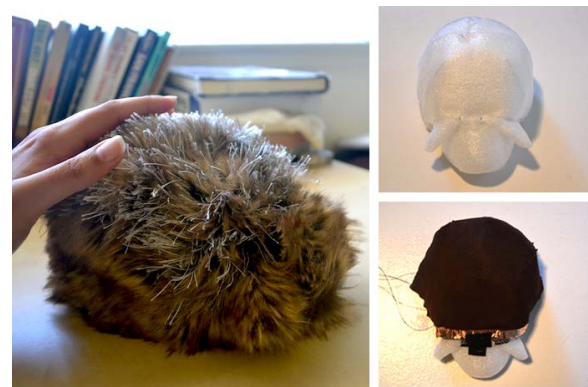
Figure 1. Complete affective touch-sensing zoomorphic prototype with pressure and conductive fur sensors (left), inner styrofoam and plastic skeleton (top right), skeleton with fabric pressure sensor (bottom right).
