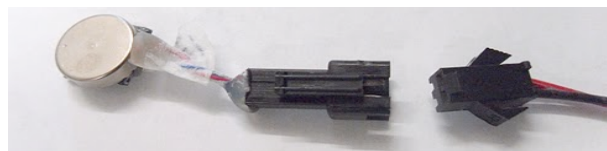
Figure 2. VPM2 eccentric-mass tactor
