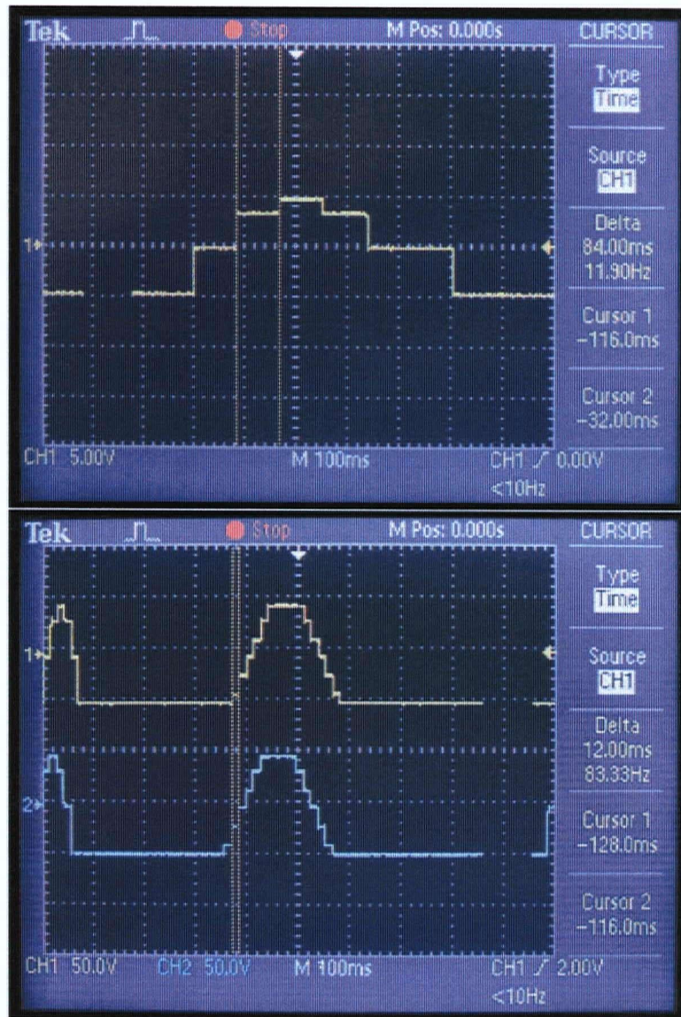
Figure 4.5: Measured outputs under conditions of load (running the browser application). Above , prior to optimization. Below , after optimization, showing two adjacent output channels at once.
