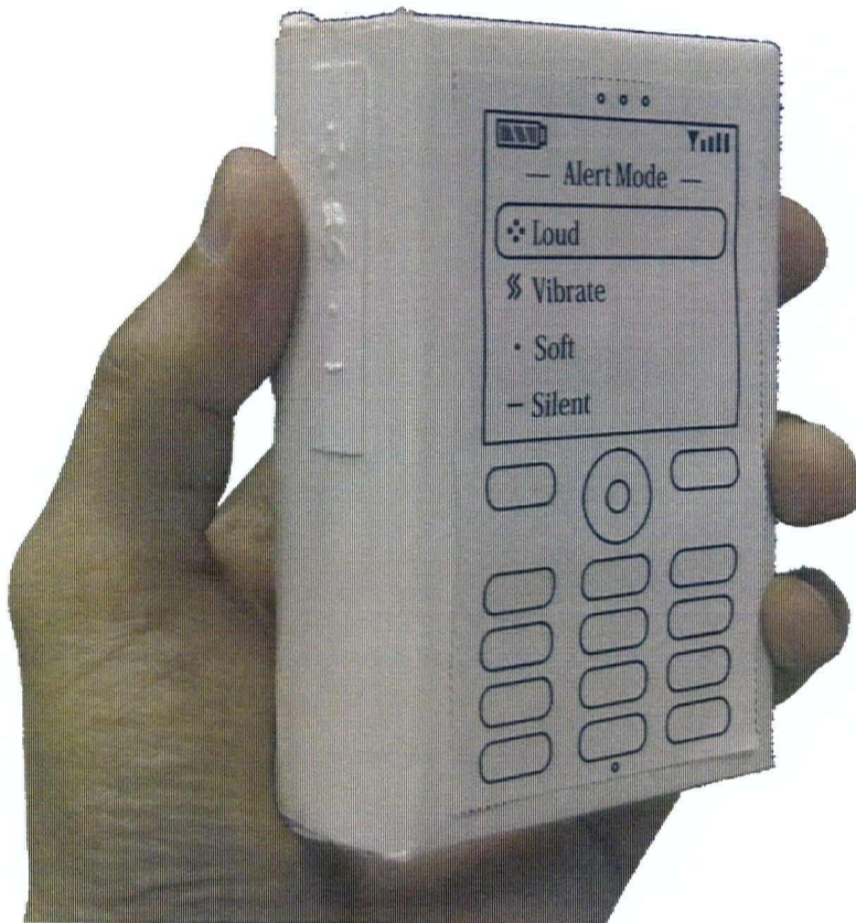
Figure 3.7: Low-fidelity foam mockup used for early user evaluation of the menu selection application concept. There is a textured plastic tactile strip mounted on the left side of the mockup.
