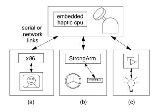
Figure 9: Embedded haptic interfaces can control arbitrary targets such as (a) an embedded x86 driving a video monitor; (b) a StrongArm controlling an automobile sound system; (c) a network of analog circuits, each responsible for one light in a room lighting system.
