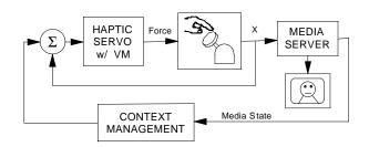
Figure 5: Inner and outer closed control loops.
