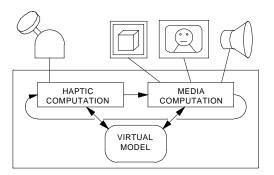
Figure 2: Single-threaded architecture
