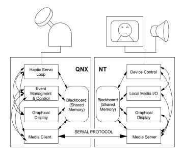
Figure 4: A two-machine instantiation of our architecture for haptic control of video. Interprocess messages are shown as curved lines; references to shared memory as straight lines.
