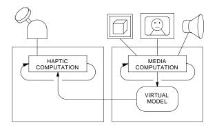
Figure 3: Multi-threaded architecture
