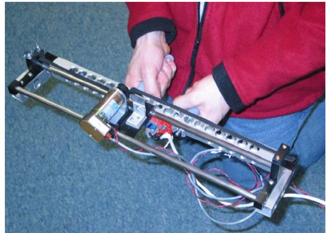
Figure 1: TorqueBAR ungrounded force feedback device
