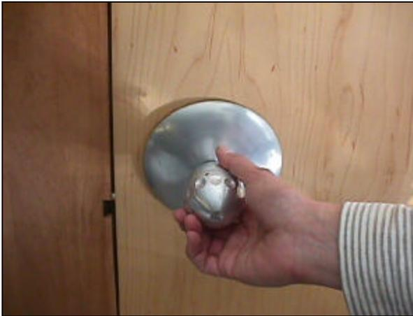
Figure 8: The Aladdin haptic door knob, which combines force feedback with a thermal display.
