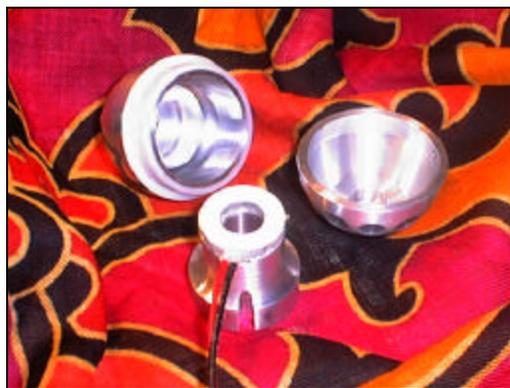
(b) disassembled to reveal the touch surface, thermoelectric module and internal heatsink.
