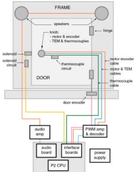
Figure 2: Prototype operational schematic.
