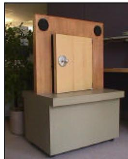
Figure 1: The Aladdin engineering prototype, shown here with the thermal knob, is a half-door with a fully functional knob, latch control and door angle sensing, and an auditory display.
