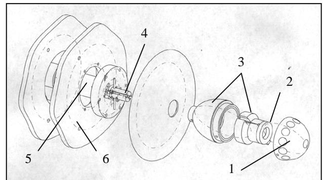
Figure 3: Exploded drawing of thermal knob, actuator and cutaway mounting in door.
