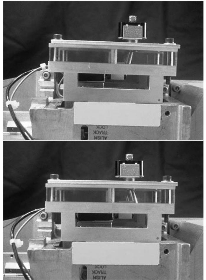
Figure 1: A force display used as a force probe. The target, a toggle switch, is inverted over the force probe. The probe has moved from left to right between the two photographs, deflecting the toggle bat.
