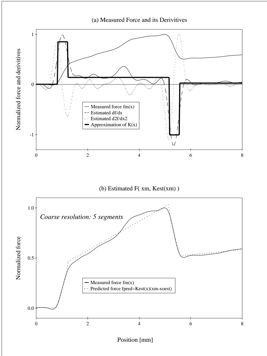
Figure 2: The identification algorithm on a stiffness-dominated system, finding zone transitions at a coarse resolution (6 transitions found). (a) Measured force as a function of controlled position ( $f_m(x_m)$ ), and derived  $\frac{d(f_m)}{dx_m}$  and  $\frac{d^2(f_m)}{dx_m^2}$ . The heavy segmented lines are regions of constant estimated  $\hat{K}(x)$ . (b) Measured force ( $f_m(x_m)$ ) and predicted output force ( $\hat{f}(x)$ ) based on estimated  $\hat{K}(x)$  and  $\hat{x}_o(x)$ .
