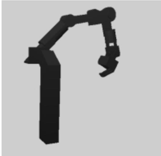
Figure 3: SARCOS arm with maximal elbow mobility.
