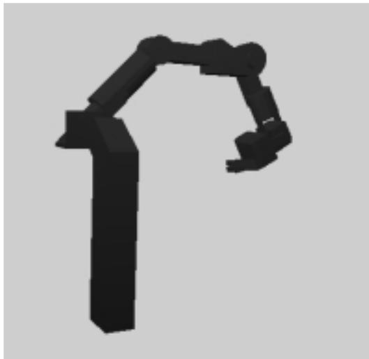
Figure 4: SARCOS arm with minimal elbow mobility.
