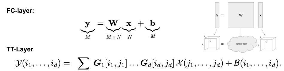
A TT-layer transforms a *d*-dimensional tensor  $\mathcal{X}$  (formed from the corresponding vector x) to the *d*-dimensional tensor  $\mathcal{Y}$  (which correspond to the output vector y). We assume that the weight matrix W is represented in the TT-format with the cores  $G_k[i_k, j_k]$ .
