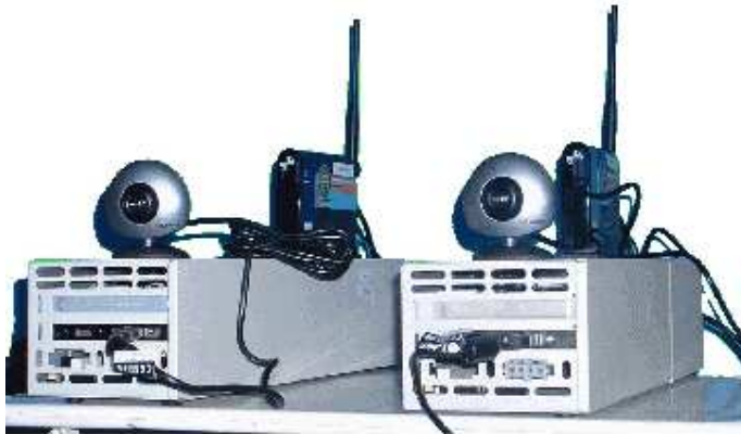
Figure 3–4: Hardware for two nodes in our Sensor Network. Images from the camera at each node are obtained using a low powered computer and are transmitted over the network using a combination of wireless and wired networking.
