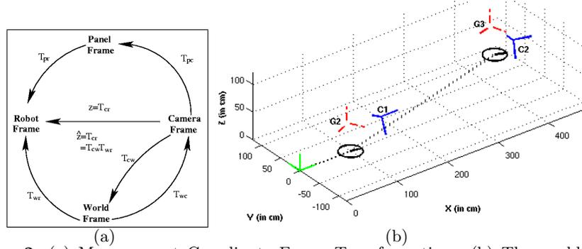
**Fig. 2.** (a) Measurement Coordinate Frame Transformations. (b) The world (at  $[0,0,0]$ ), robot (denoted by a circle and a line for the orientation), target grid (dashed lines G1,G2) and camera (solid lines C1,C2) coordinate frames. The trajectory of the robot is marked by a dotted line.
