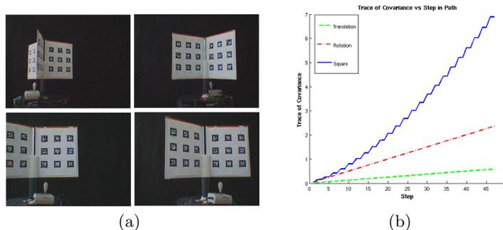
**Fig. 3.** (a) Sample Images from Square Pattern. (b) Odometry Error Accumulation for 3 Local Calibration Paths
