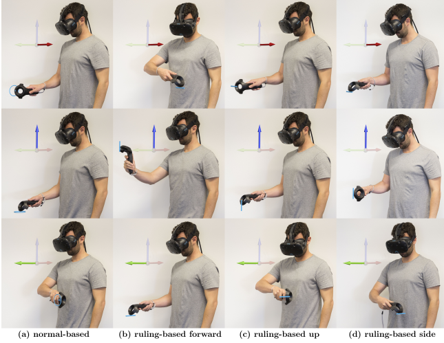
Figure 6: (a) Mapping the three major drawing planes (front facing, side facing and horizontal) to corresponding hand-held controller orientations using normal brush. (b-d) Wrist twist minimizing hand and controller orientations necessary to align a local controller axis (b - forward, c - up, d - side) with each of the major global axes (up, side, front).
