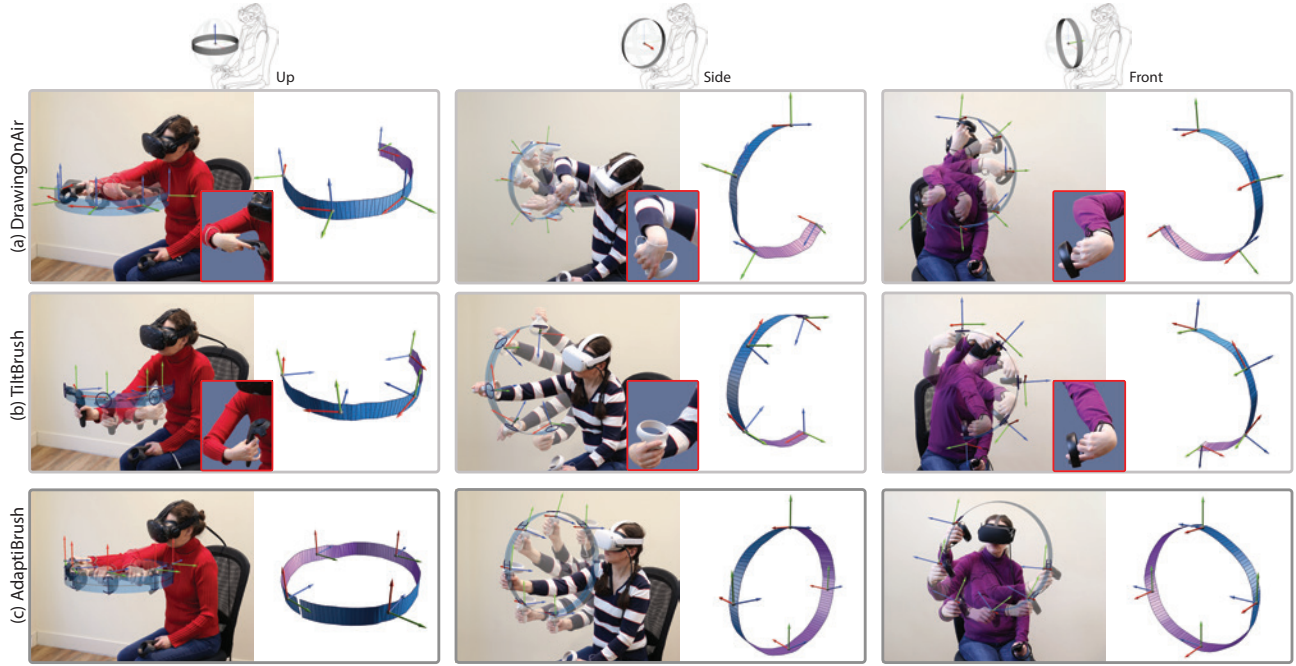
Fig. 5. Cross-product based brushes (a) [Keefe et al. 2007], (b) [TiltBrush 2019] force users to twist their wrists into awkward positions to smoothly change ribbon normals, making curved ribbons challenging to draw and preventing users from drawing even medium complexity curved ribbons such as cylinders. Using AdaptiBrush, users can draw curved surfaces such as cylinders while keeping their wrist orientation fixed for any choice of cylinder axis (c). Columns left to right: HTC Vive, Oculus Quest 2, and Oculus CV1. See supplementary video for complete motions.
