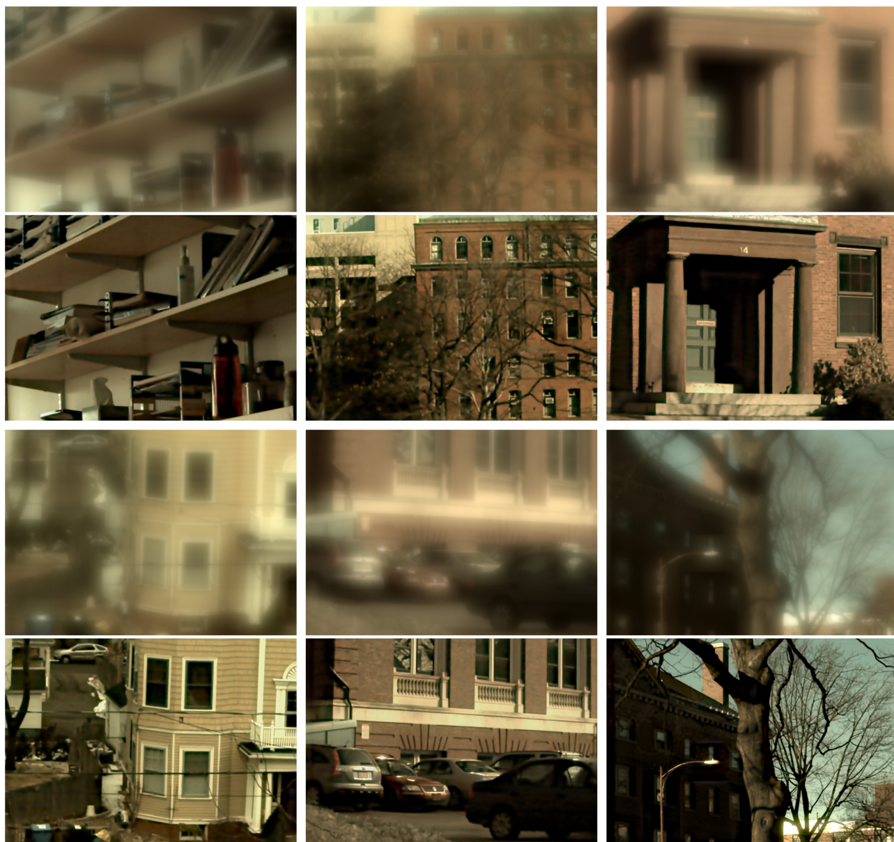
Figure 6: Blurred and deblurred results of selected synthetic scenarios from hyperspectral dataset [Chakrabarti and Zickler 2011; Skauli and Farrell 2013], with \sigma = 0.005 Gaussian white noise added.
