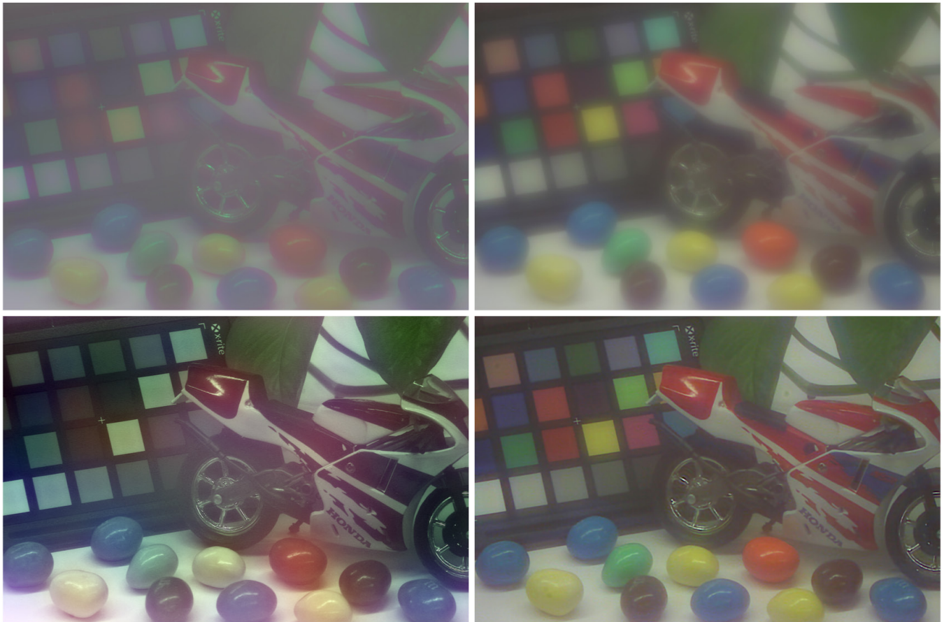
Figure 8: Comparison of a Fresnel lens (left column pair) and a diffractive achromat (right column pair), with their blurred and deblurred results of natural scenarios. Both are captured at same depth with single exposure under same indoor artificial and mixed illumination, using a single 0.5mm ultrathin Fresnel phase plate and a diffractive achromat we have fabricated, respectively. Note that for the Fresnel one, a preliminary color calibration is added using Adobe Photoshop application. From which we see that although blur has been mostly removed for the Fresnel lens one, considerable color artifacts are observed, explicitly illustrated by the failure of recover blue and red colors. On the contrary, the recovery from our diffractive achromat successfully removes the blur, as well as preserve the color fidelity.
